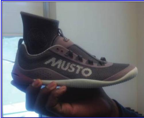
A full-color shoe concept model printed with 3D Systems' ColorJet technology.
